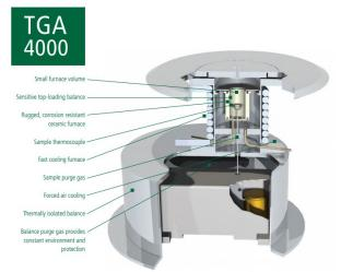
In Thermogravimetric Analysis (TGA), the mass of a sample is measured over time as the temperature changes. This provides information about phase transitions, decomposition, absorption and desorption as well as chemical phenomena.
