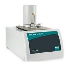
Heat flux DSC is of a single furnace design with a temperature sensor for each of the sample or reference pans located within the same furnace. When transitions in the sample are encountered, a temperature difference is created between sample and reference.
